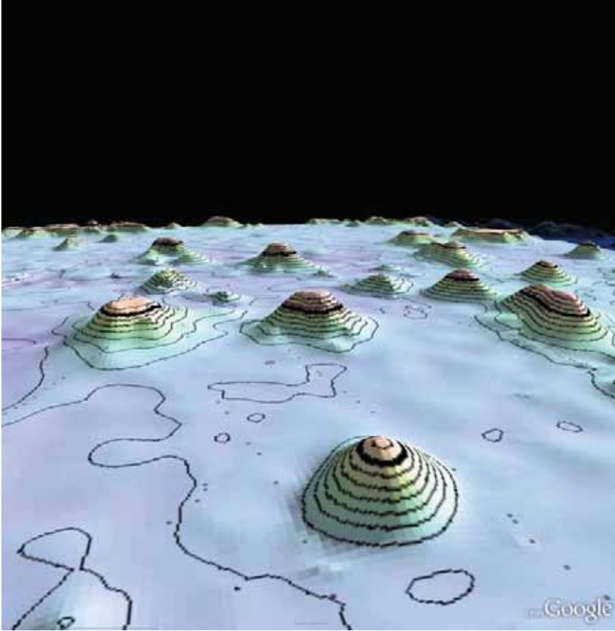
Figure 1. Bathymetry of large seamounts in the western Pacific based on a new global bathymetry grid (SRTM30_PLUS). This grid provides the ocean base later for Google Earth. Contour interval is 500 m.
