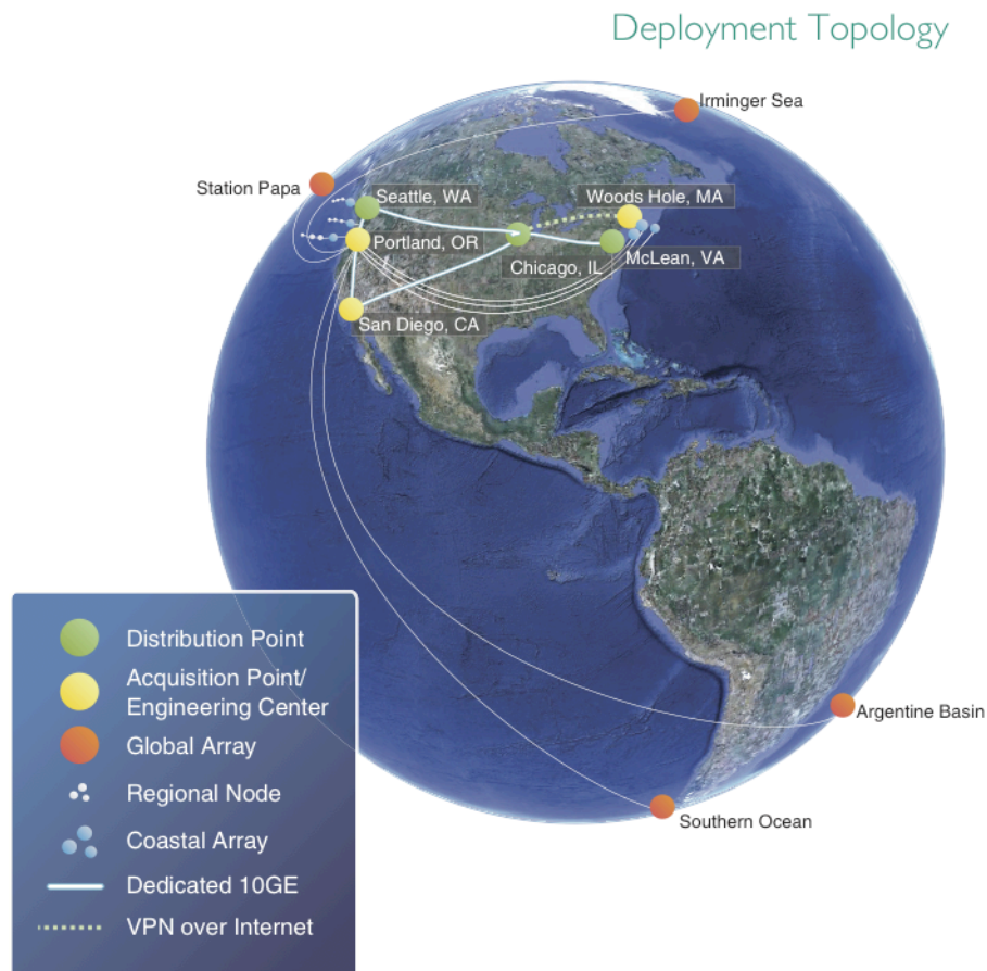
Figure 1: The OOI networks connecting platforms (e.g. buoys, autonomous vehicles, and seafloor cabled nodes) and sensors (e.g. seismometers, pH instruments and cameras) in the OOI. The primary continental network connects Seattle, Chicago, San Diego and Portland through a 10GE network in a triangular geometry which supports data transport from the primary acquisition point in Portland with the remainder of the network. The loss of a single connection or node in the network doesn't affect data flow. The design reliability of the network is 99.999%.
